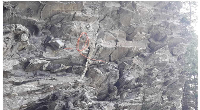
Rock cliff monitored by Huggenberger with a Piconode
