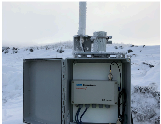
The battery-powered data loggers, installed in a major iron ore mine in Quebec, where temperatures may drop to -40°C.
