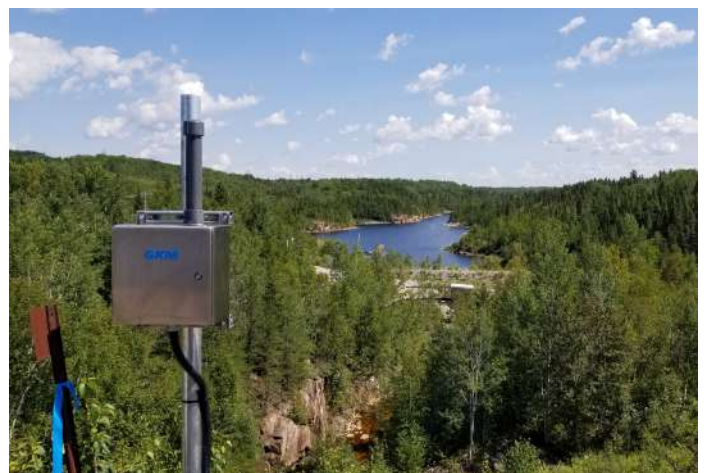
Single channel vibrating wire node in heavy duty enclosure
