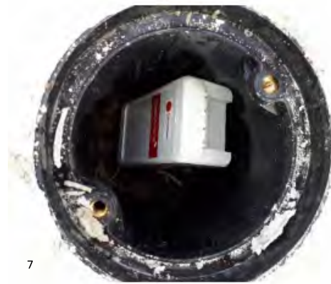
Figures 7 and 8: Data loggers connected to piezometers around the shaft and TBM alignment
