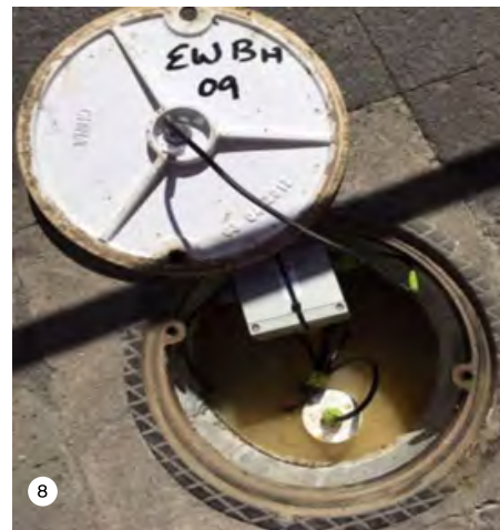
Figures 7 and 8: Data loggers connected to piezometers around the shaft and TBM alignment
