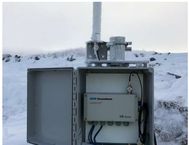
The battery-powered data loggers, installed in a major iron ore mine in Quebec, where temperatures may drop to -40^{\circ}\text{C} .
