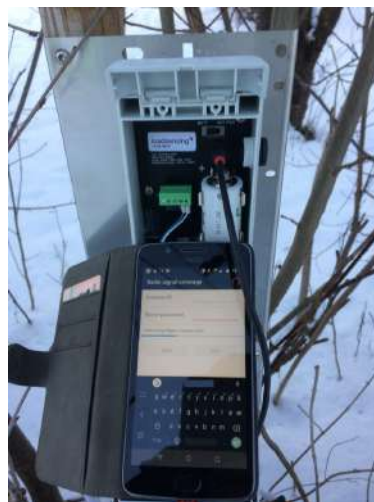
Worldsensing data node being configured simply through a mobile application
