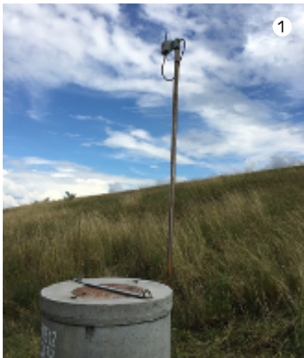
1 - A Loadensing vibrating wire 1-channel logger connected to a vibrating wire piezometer.
