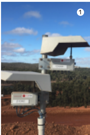
1 - Loadsensing Vibrating Wire 5-channel data logger installation
